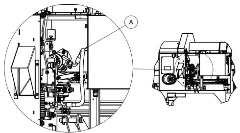
• Remove the hydraulic hose marked A in the picture above.
