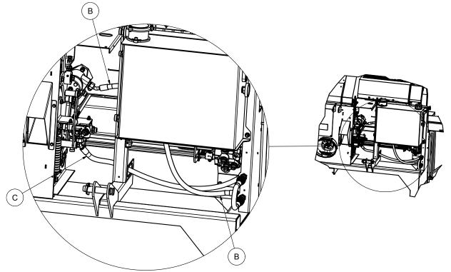
• New hydraulic hoses B and C must be connected as shown in the picture above.
